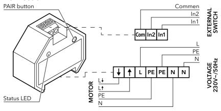
The receiver can be controlled by an external switch. This must be potential-free. Under no circumstances must 230 V be connected via this input; this would destroy the control unit! We recommend using switches with gold contacts.
